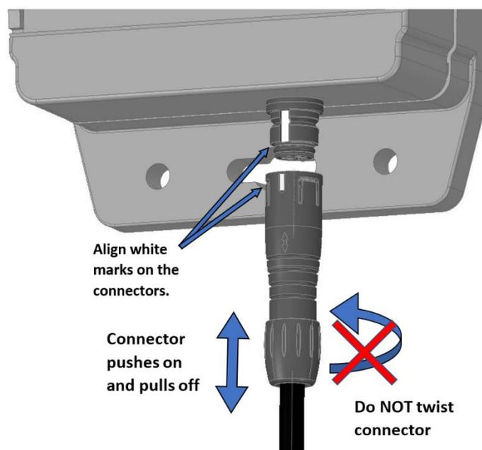
Figure 2 Temperature Probe Connector
