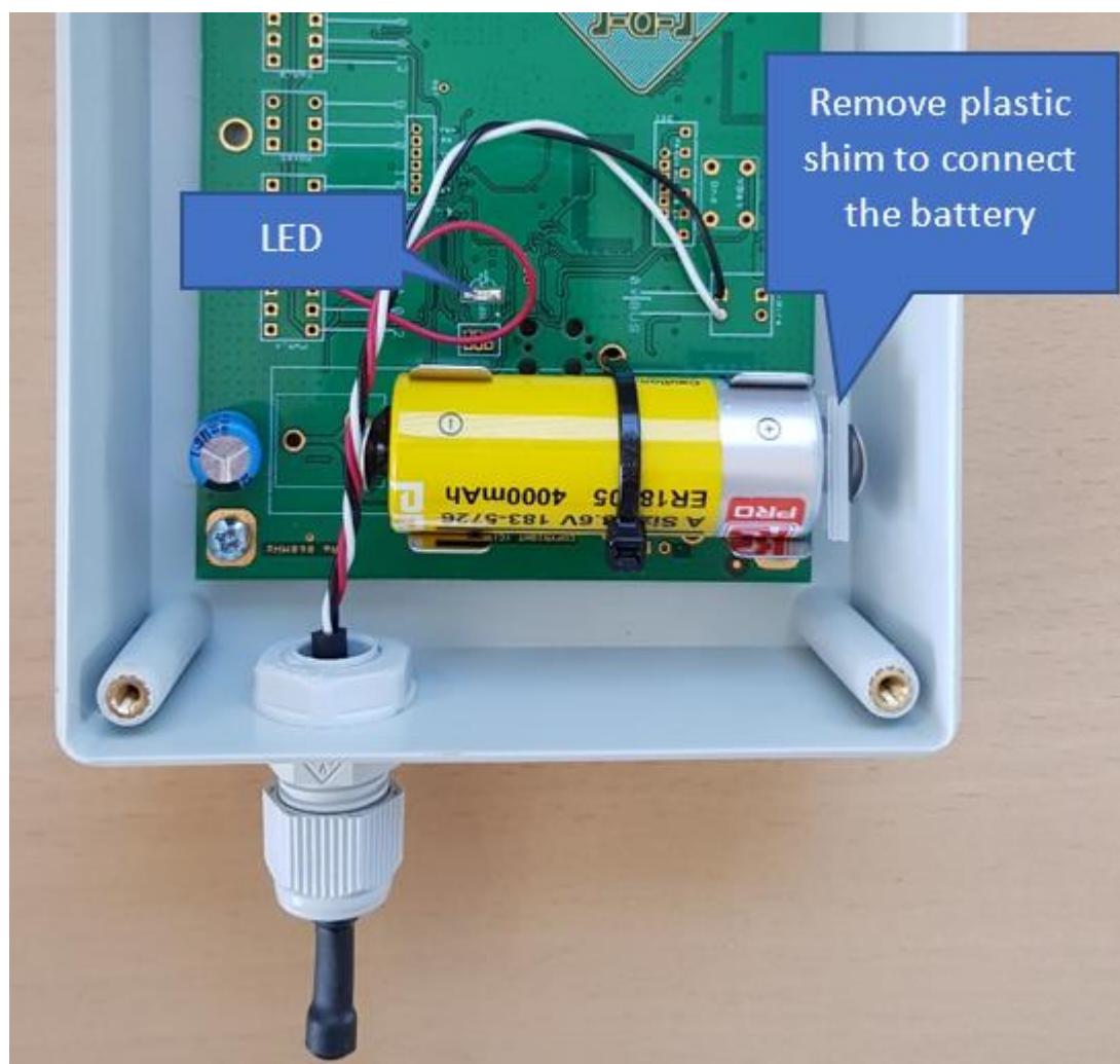
Figure 2 Inside of node showing position of plastic shim.
