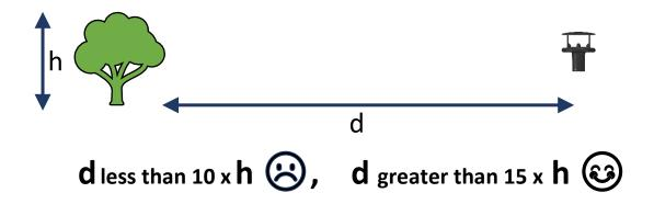
If possible, the sensor should be at a distance of least 10 times the hight of an object like a tree or building from that object.
