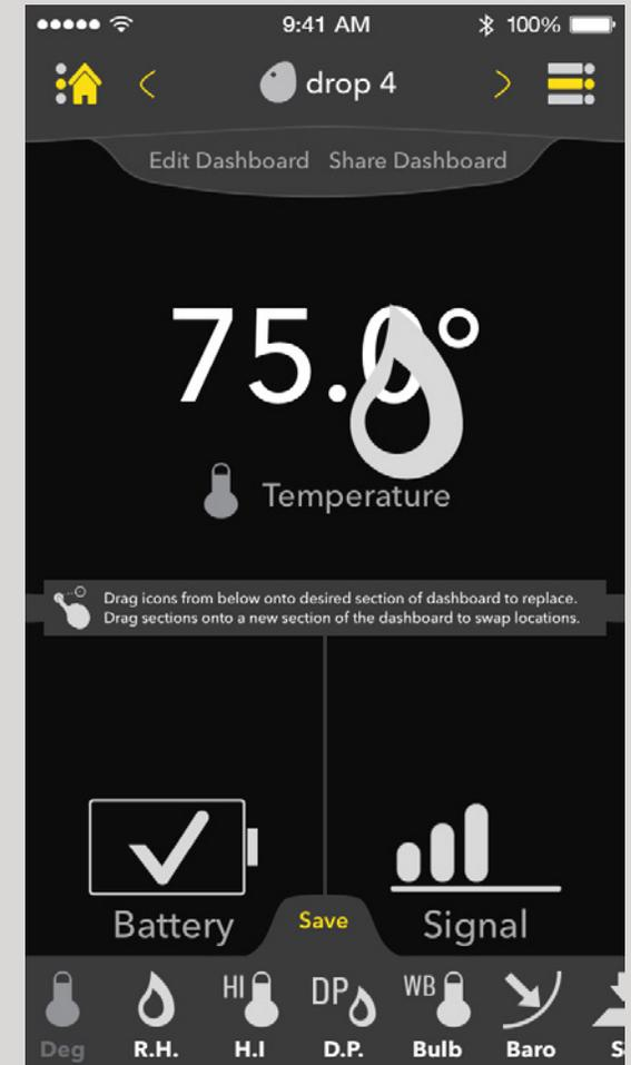
When the user drags the icon to a section of the dashboard, a large icon will follow the dragging motion. Measurements can also be switched from panel to panel within the edit screen by dragging one measurement from one panel to the other desired panel.
