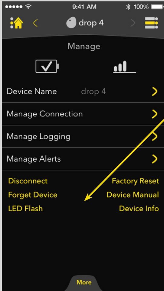
Disconnect: Removes active connection between the app and device
