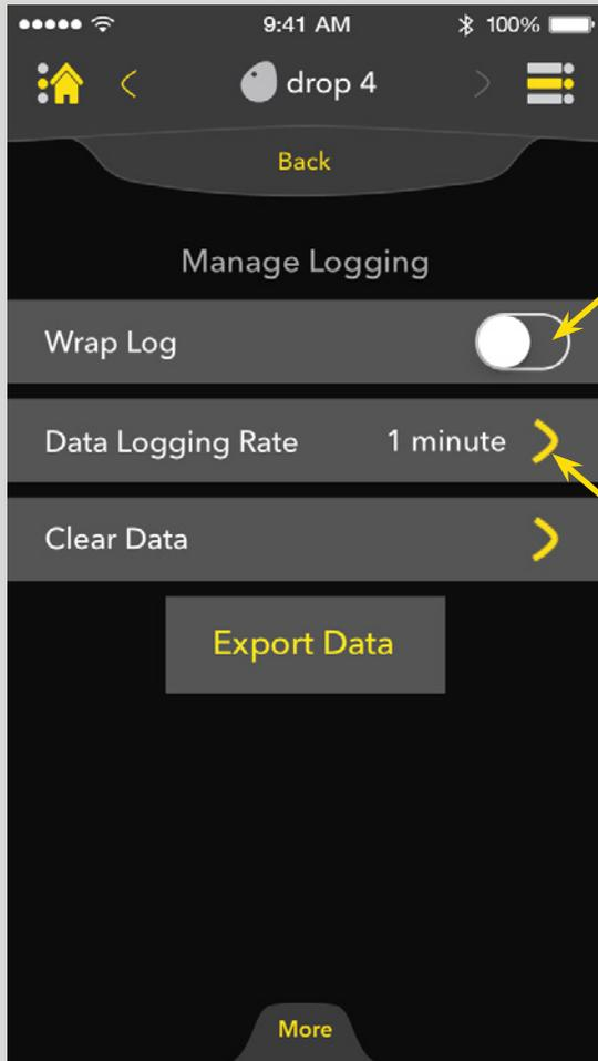
Wrap log is an overwrite feature that will discard the oldest data point to capture new data when the log becomes full.
