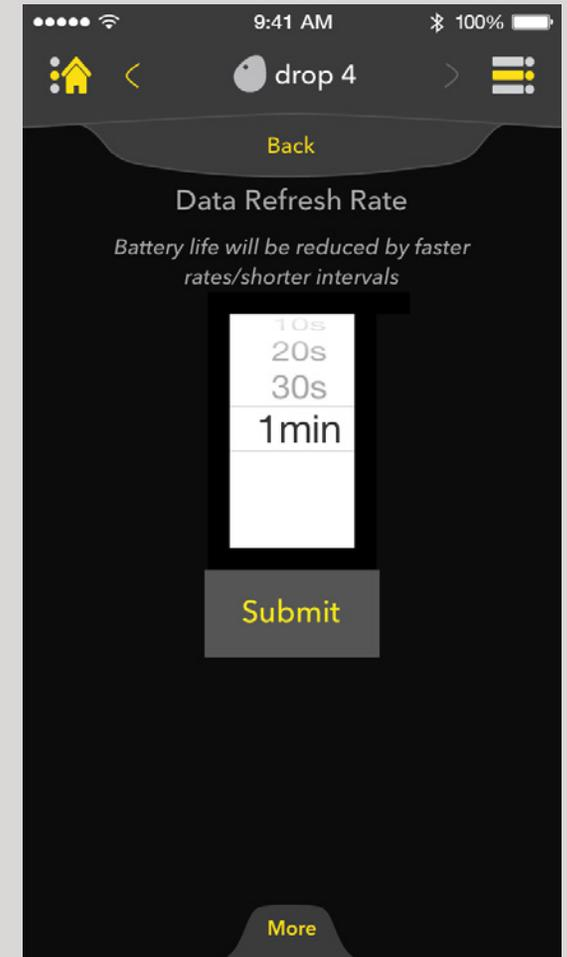
Data Refresh Rate can be altered by using the scroll wheel to adjust the rate and then clicking submit to confirm the change.
