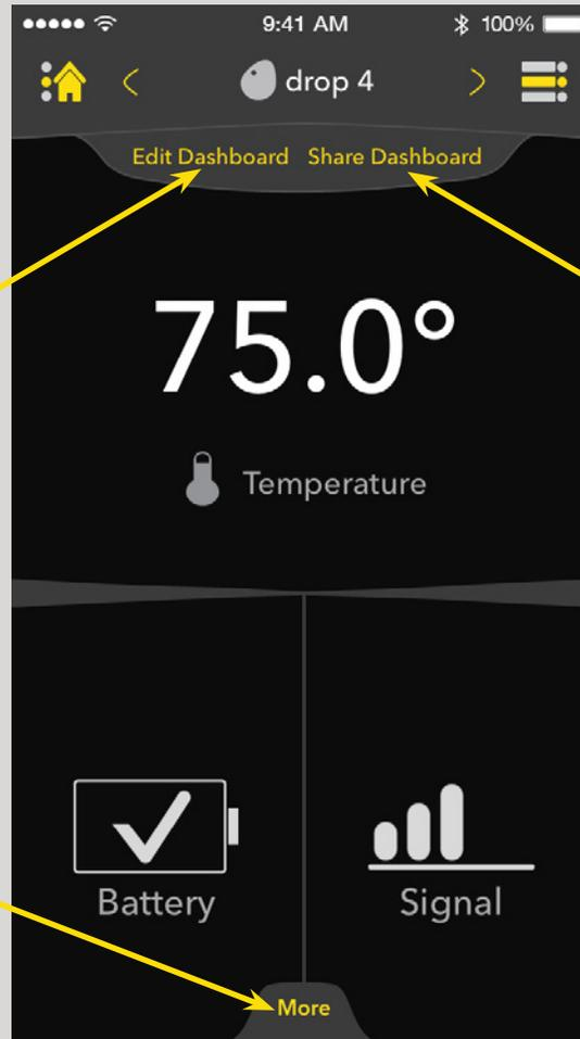
The Edit Dashboard option allows the user to replace the current measurements with new measurements and re-arrange measurements on the dashboard.
