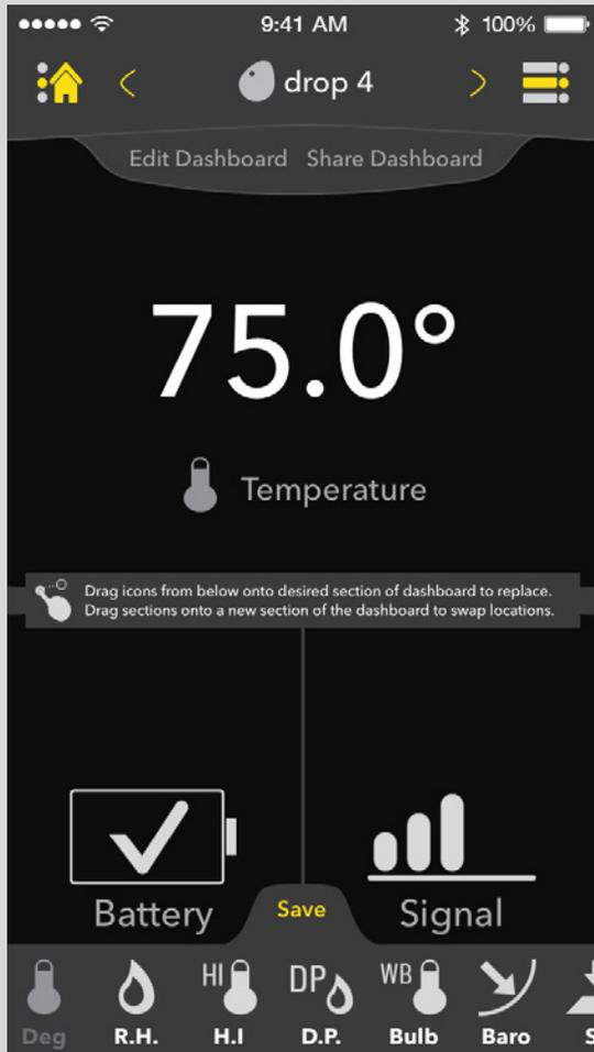
Once Edit Dashboard has been selected, the edit menu appears at the bottom of the screen displaying the different measurements available for the device currently being viewed.
