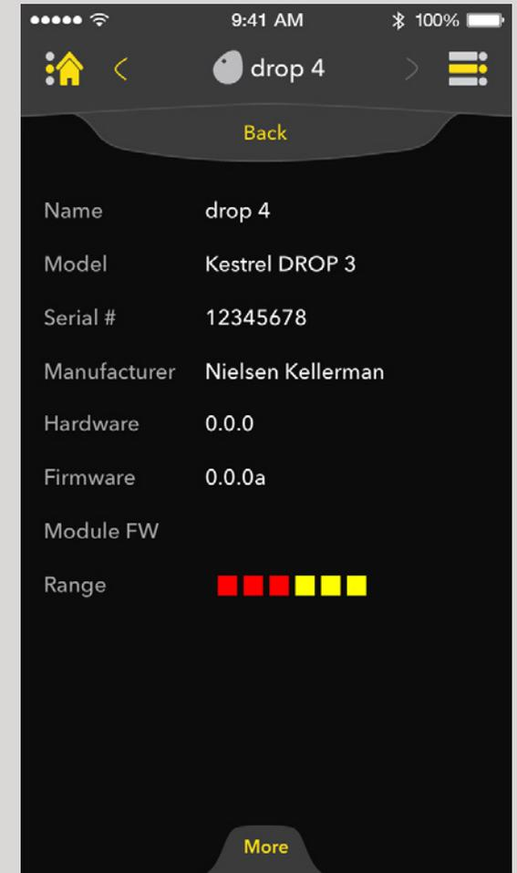
Within the Device Info option the user can view the device's model number, serial number, manufacturer, hardware version, firmware version as well as the range when connected.
