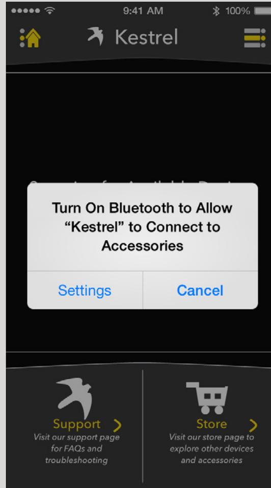
If Bluetooth is turned off on the device, a prompt will appear asking to turn Bluetooth on. With Bluetooth off the app will not be able to connect to Kestrel devices.
